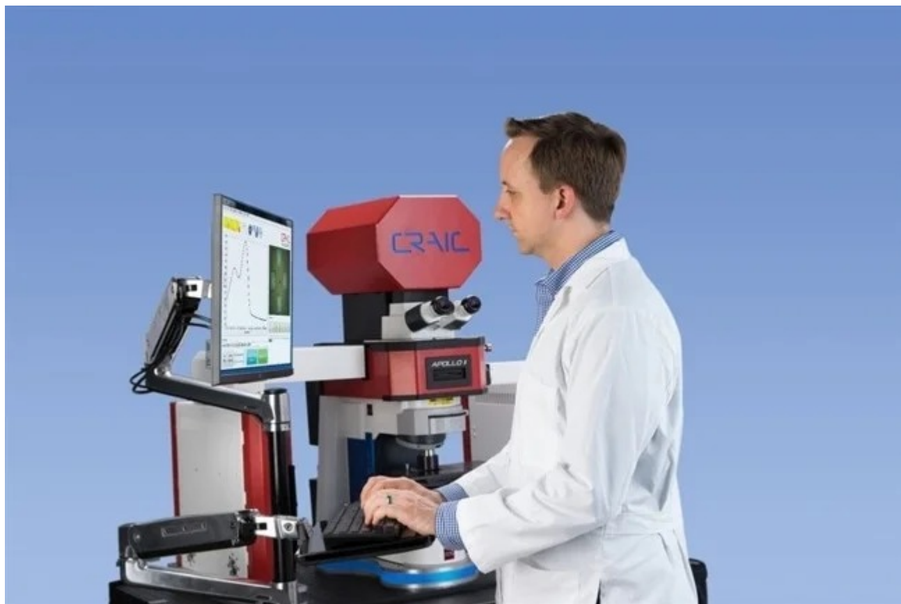
Figure 1. The 2030PV PRO™ UV-VIS-NIR microspectrophotometer from CRAIC Technologies. This instrument can be configured for transmission, reflectance, fluorescence, photoluminescence and Raman spectroscopy and imaging
