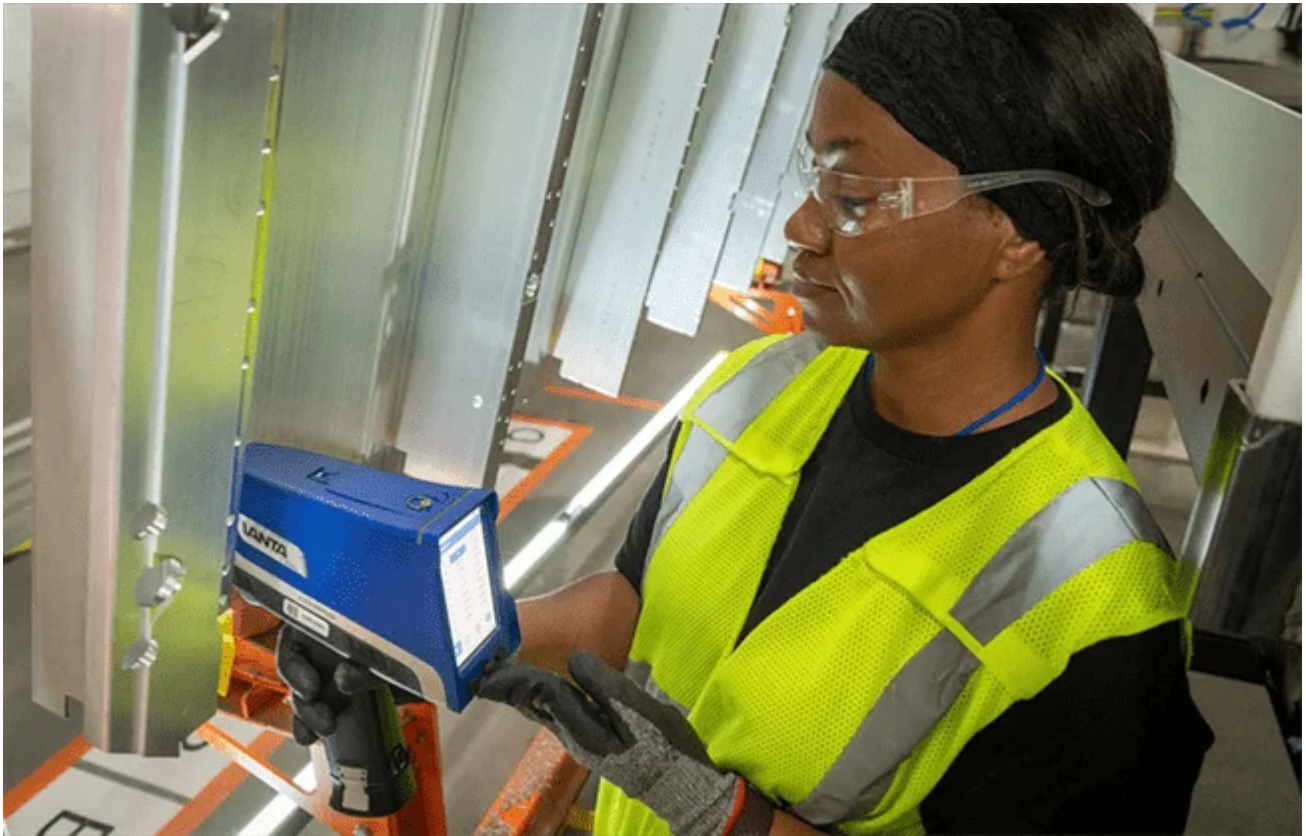
A technician performs coating analysis using a handheld XRF analyzer. Image Credit: Evident Corporation (XRF / XRD)
