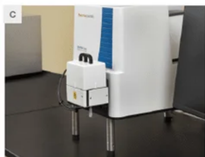
Figure 1. A) A view of the DXR3 Flex Raman Spectrometer with labelled features. B) The microscope sampling accessory. C) The macro sampling accessory. D) The fiber probe sampling accessory. Image Credit: Thermo Fisher Scientific – Chemical Analysis
