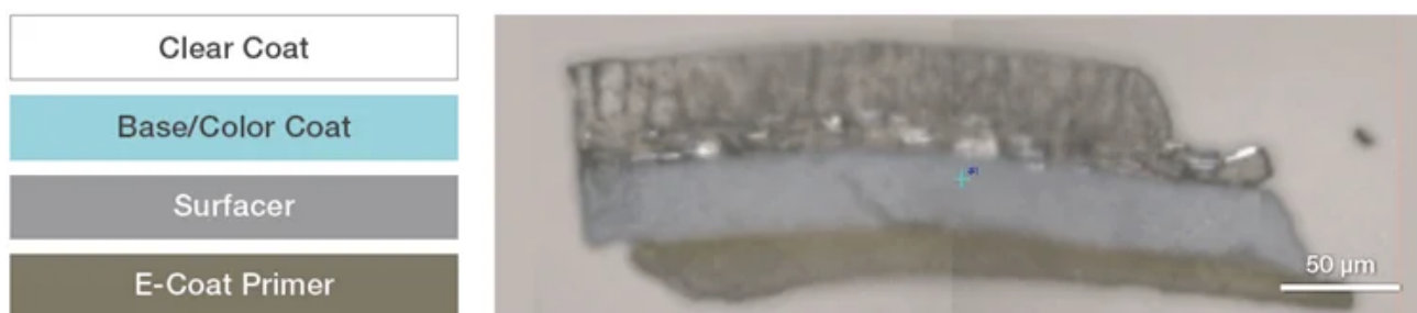
Figure 1. Schematic of a typical four-layer automobile paint sample (left). Video mosaic image of a paint-chip cross-section taken from the door of an automobile (right). Image Credit: Thermo Fisher Scientific – Materials & Structural Analysis
