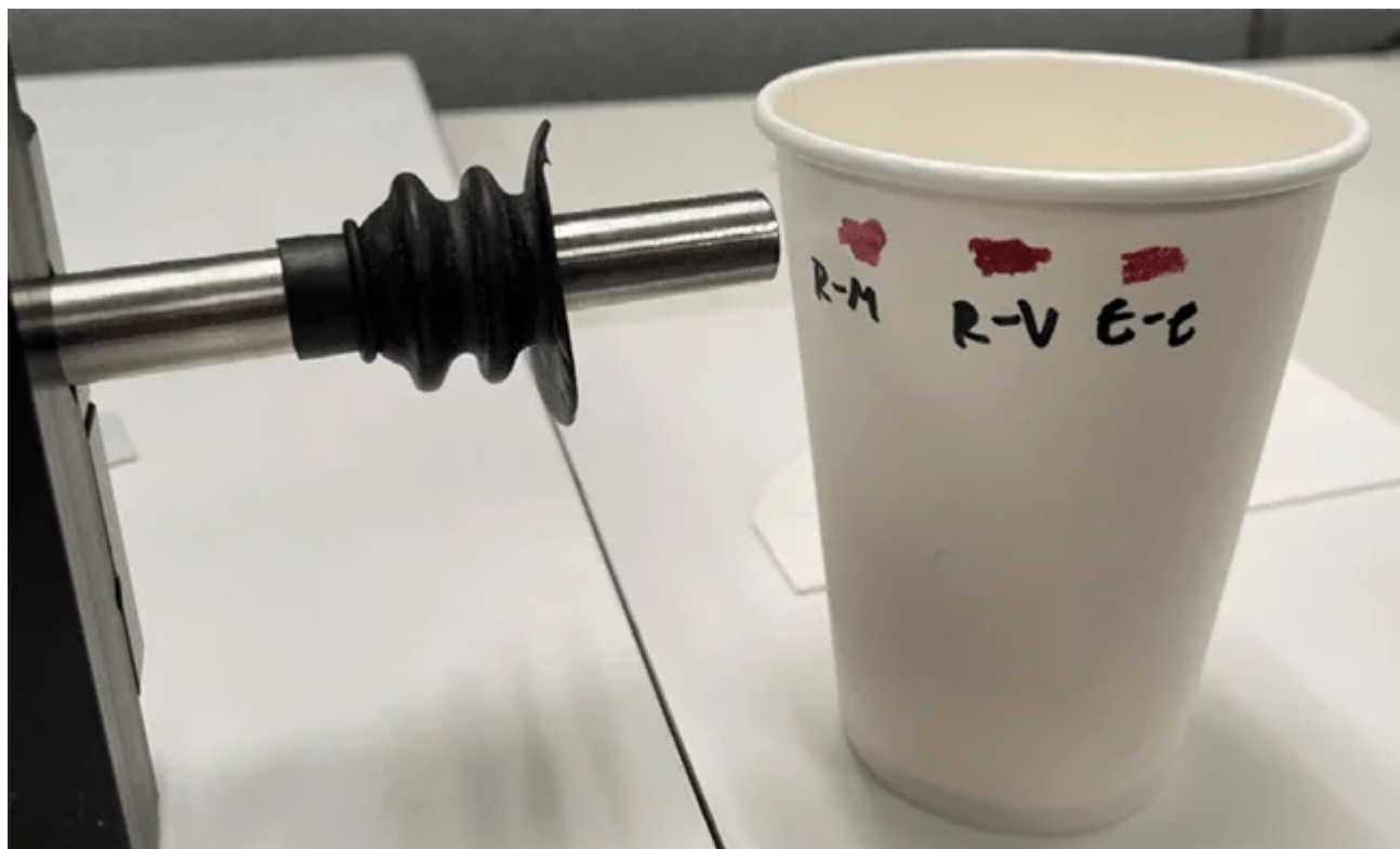
Figure 5. An in situ measurement of lipstick on a cup through the fiber probe accessory. Image Credit: Thermo Fisher Scientific – Chemical Analysis
