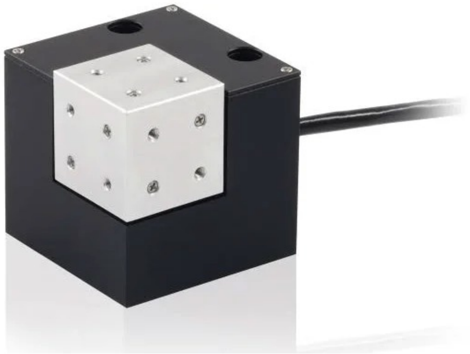
Fig 4. NanoCube ® , piezo-based, high dynamic, 3-axis scanner with 100 \mu\text{m} travel range. Besides its nanoscale resolution and blazing speeds, this flexure-based subsystem can perform continuous tracking without wear. Image Credit: PI (Physik Instrumente) LP
